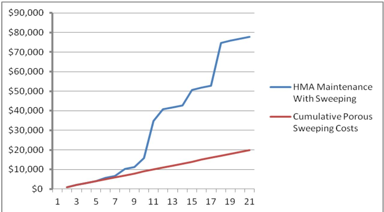
And how did we come up with this information? Due to space limitations, the details don't fit here, but our Congress presentation details a typical maintenance cycle with costs totaling some \$57,750 over 20 years for crack sealing, patching, and other typical maintenance on a 36' wide residential street. Any member can view this presentation under the electronic postings for Congress sessions. Or come and see us in Chicago at 8am on August 25<sup>th</sup>.
