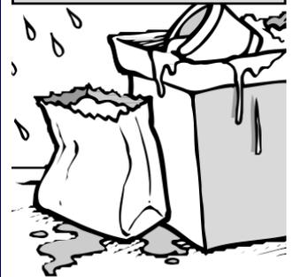
*Keep trash covered to prevent exposure to rain which can cause overflows of materials onto the ground and into storm drains.*
